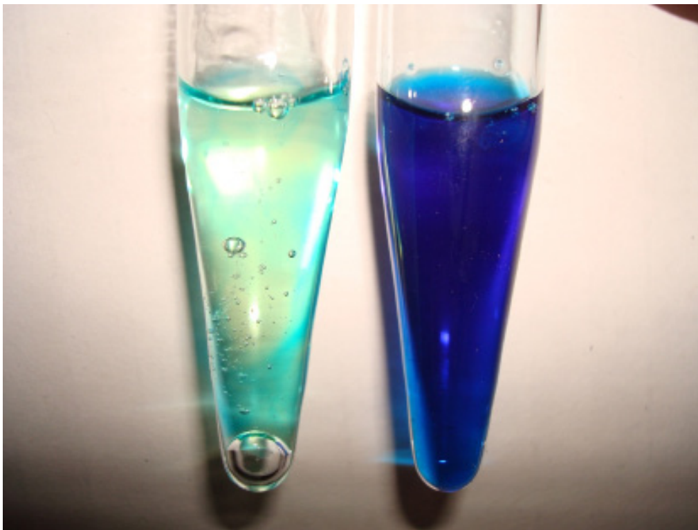
Figure 4: Photographs of thin and thick egg white fractions separated by filtration. Two mls of methylene blue were added to the egg white of a single egg which was then added to the filter surface. The fraction that passed through the filter was dark blue (Fig. 4 right) while the fraction on the filter surface was almost colorless (Fig. 4 left).
