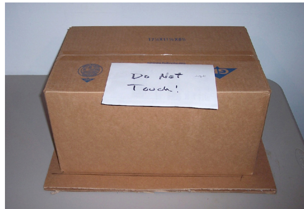
Figure 5. The Cardboard Control Enclosure. It must be placed on a thick cardboard sheet, to insulate against possible dielectric or metallic influences from the table upon which it sits.
