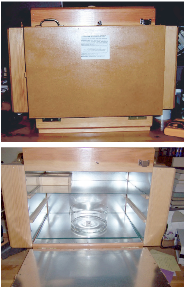
Figure 4. The ORAC-Charger Enclosure used for these experiments. The door for the ORAC opens downwards in this design.
